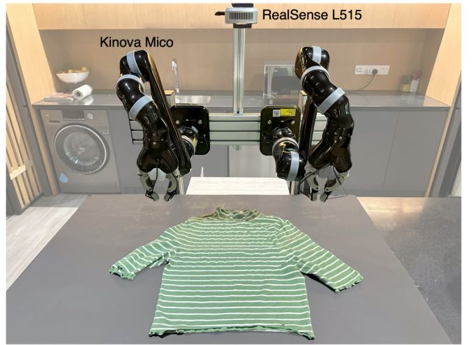
Fig. 4: Setup for real-robot experiments. The dual-arm system consists of an Intel RealSense camera for depth sensing and two Kinova Mico arms.
