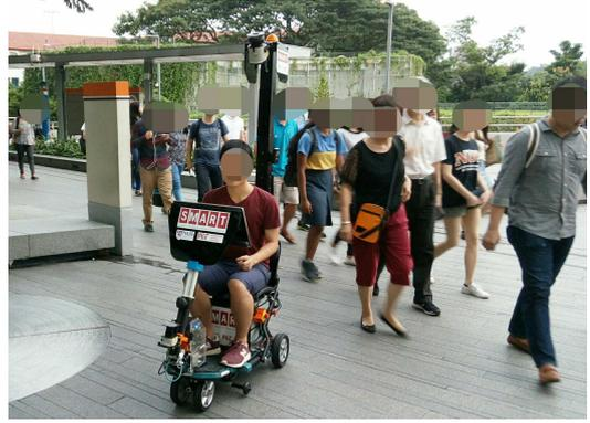
Figure 7: Our single-seater autonomous vehicle, *Scooter*, driving amidst pedestrians.
