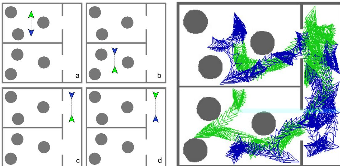
Figure 3.8. Test scene 4 for the wheeled robot carts. The environment consists of two rooms that contain large circular obstacles and are connected by a narrow hallway.
