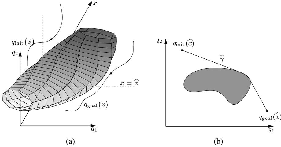
Figure 5.2. The base placement problem in the configuration space. The robot is a two-dof planar arm with joint angles  $q_1$  and  $q_2$ . The base of the robot lies on a line parameterized by  $x$ . (a) Schematic drawing of the configuration space of the robot base and joints. Shaded parts indicate obstacles. (b) Cross section for the optimal base location  $\hat{x}$ . It contains the optimal path  $\hat{\gamma}$ .
