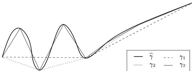
Figure 2.10. Piecewise linear approximations to a smooth path. The paths  $\gamma_1, \gamma_2, \gamma_3$  are three-, five-, and nine-vertex piecewise-linear paths approximating  $\hat{\gamma}$ . In the right portion of  $\hat{\gamma}$ , all approximations are reasonably good, while in the left portion of  $\hat{\gamma}$ , only  $\gamma_3$  approximates  $\hat{\gamma}$  well.
