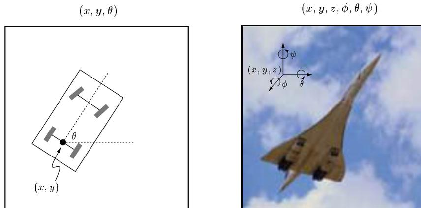
Figure 2.1. The configuration of a rigid body.
