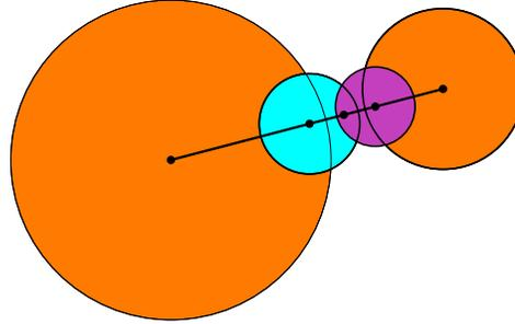
Figure 2.7. Recursively bisecting the straight line segment into two segments until the collision-free spheres centered at the endpoints of segments cover the segments completely or one endpoint is in collision.
