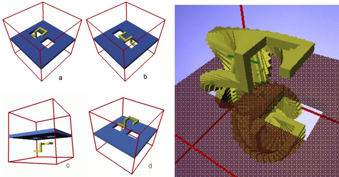
Figure 2.18. Test scene 3 for rigid bodies: a snake-shaped object passing through the small holes in the obstacle.
