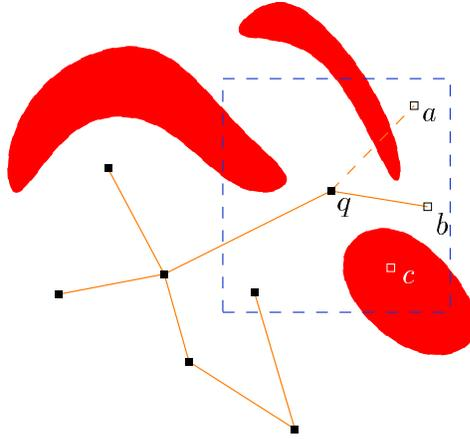
Figure 2.6. Adding a new milestone. The configurations  $a$  and  $c$  are rejected, but  $b$  is accepted as a new milestone.
