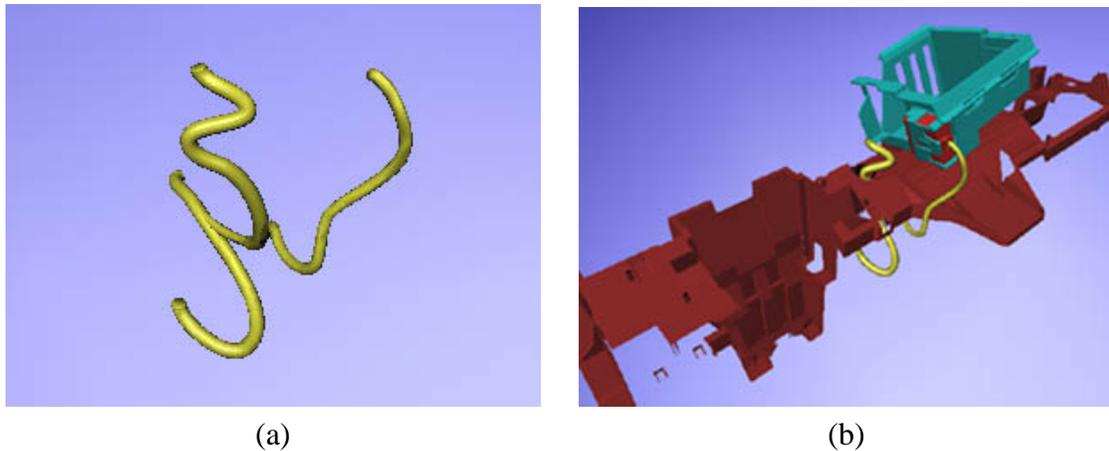
Figure 2.19. An example of assembly maintainability checking. (a) The part to be removed. (b) The part in the installed position.
