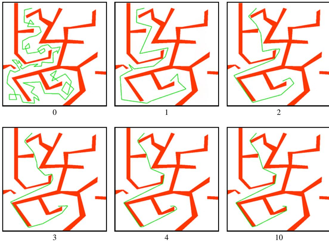
Figure 2.9. Minimum-length paths computed by ADAPTIVE-SHORTCUT after 0, 1, 2, 3, 4, and 10 iterations.
