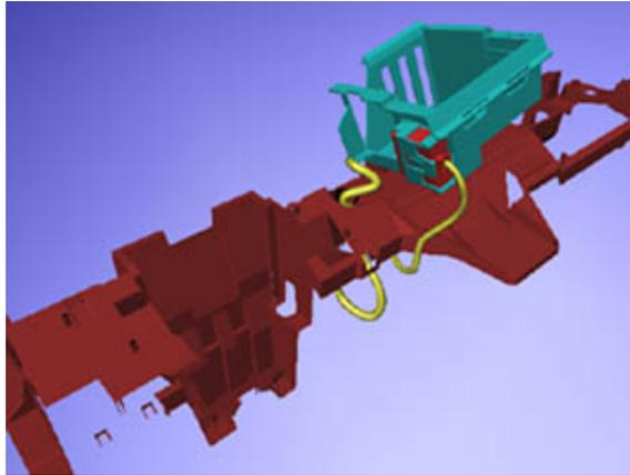
Figure 1.1. Assembly maintainability checking, whose goal is to remove a specified component from an assembly of mechanical parts without collision.
