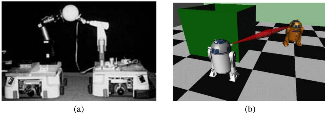
Figure 3.3. Two-cart non-holonomic robots. (a) Cooperative mobile manipulators. (b) Two wheeled non-holonomic robots that maintain a direct line of sight and a distance range.
