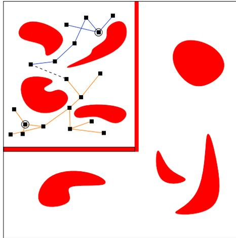
Figure 2.5. A roadmap for a single-pair problem in the 2-D configuration space. The two circles mark  $q_{\text{init}}$  and  $q_{\text{goal}}$ .
