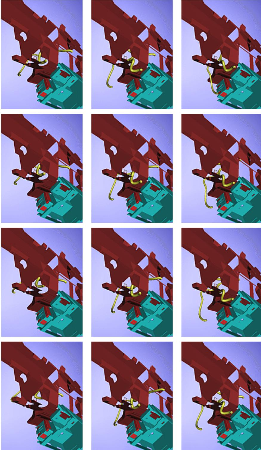
Figure 2.20. A collision-free path for removing the pipe.
