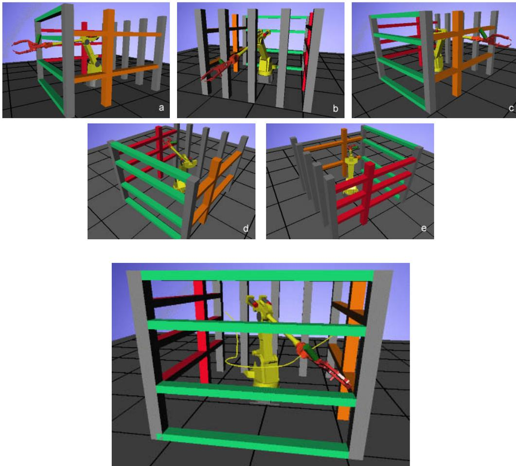
Figure 2.12. Test scene 3 for articulated objects. The horizontal and vertical bars acting as obstacles restrict the movement of the FANUC-like robot, which has a large end-effector.
