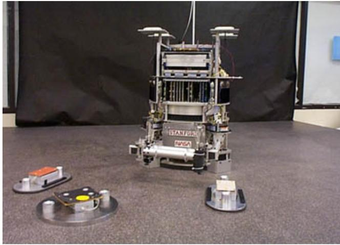
Figure 3.14. The air-cushioned robot among moving obstacles.
