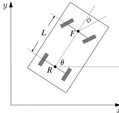
Figure 3.1. A simplified model for a car-like robot.
