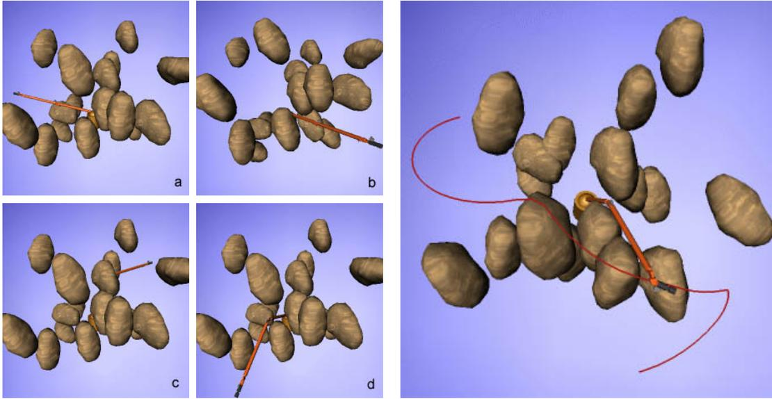
Figure 2.13. Test scene 4 for articulated objects. The skinny robot manipulator arm passes through narrow spaces between the obstacles.
