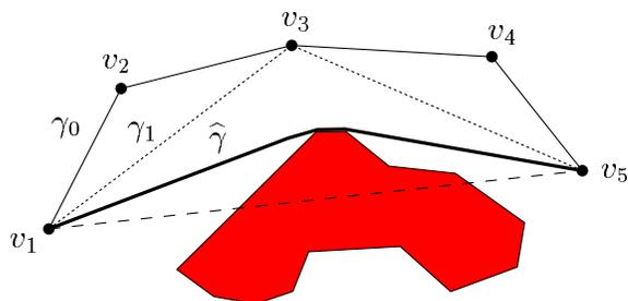
Figure 2.8. SHORTCUT gets stuck at  $\gamma_1$ , which is far from the minimum  $\hat{\gamma}$ . The path  $\gamma_0$  is the input to SHORTCUT, and  $\gamma_1$  shows the path after one iteration.
