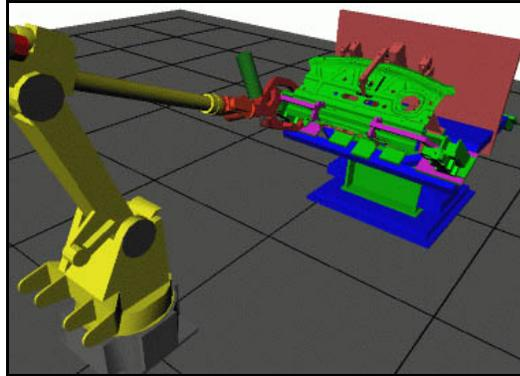
Figure 5.1. A robot spot-welding the side-panel of a car. It has to maneuver among fixturing devices and reach underneath the side-panel in order to access weld-points.
