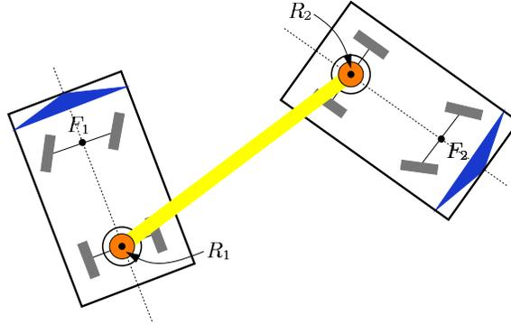
Figure 3.4. A planar model of the two robot carts.
