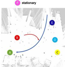
Fig. 6. A top-down view of the plaza area with a map built from LIDAR data. “A”–“F” indicate pedestrian intentions. The blue and the orange lines roughly correspond to the vehicle and the pedestrian paths, respectively, for the test run in Fig. 5.
