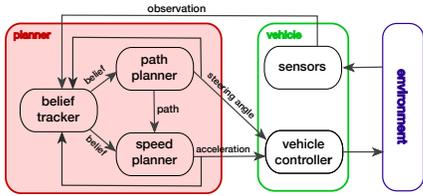
Fig. 3. Two-level POMDP-based planning for autonomous driving.
