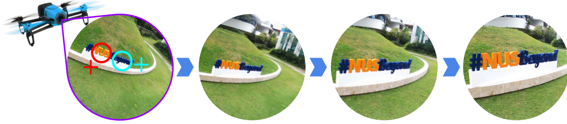
Figure 8: The viewpoint changing process. LEFT : In the initial viewpoint, each colored circle annotates an object that is composed to the position indicated by the same colored cross. MIDDLE-LEFT : The viewpoint rotates to compose one object first. MIDDLE-RIGHT : The viewpoint moves so that the other object gradually converges to the desired composition. RIGHT : The final viewpoint.
