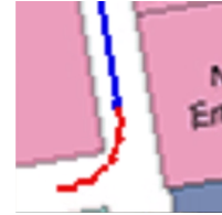
Figure 2: The LPE intention represented as a 224 \times 224 image. It captures information on the path that the robot has recently traversed (in red), the path ahead (in blue), the robot’s current position (where the red and the blue paths meet), and the local geometric environment according to the map.
